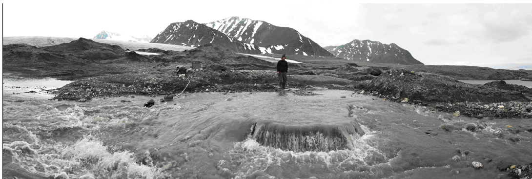
Fig.4. Upwelling water at Werenskioldbreen, location W1, July 2007, radon concentrations 8 Bq/L. The continuous measurement device can be seen, before destruction by an outburst. In 2009 and 2010 the measuring setup was put directly into the outflow.
